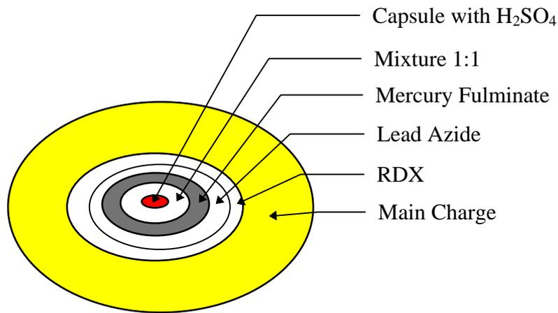
**Figure 7: Capsule timer detonator -done**
