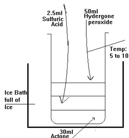
5 when the whole crystals will formed, filter them and then first wash them with water and then with 2% sodium carbonate ( $\text{Na}_2\text{CO}_3$ )
